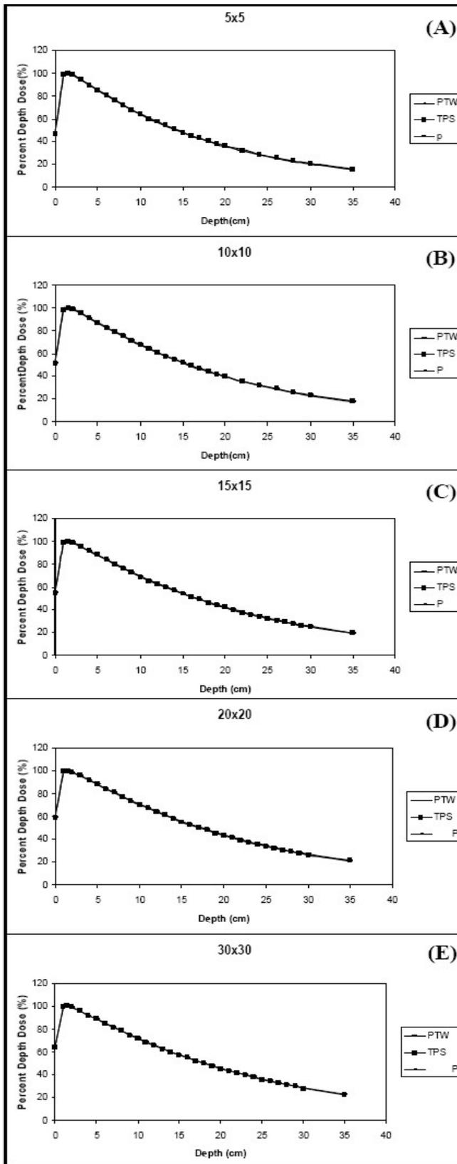
Figure 9 : Measured PDD for 6 MV photon beam emerged from Elekta Precise™ linac. at FSD =100cm in water phantom, compared with calculated and published<sup>[7]</sup> PDD. of open square field size: (A) 5x5 cm<sup>2</sup>, (B) 10x10 cm<sup>2</sup>, (C) 15x15 cm<sup>2</sup>, (D) 20x20 cm<sup>2</sup> and (E) 30x30 cm<sup>2</sup>.
