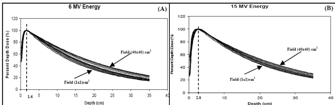
**Figure 1 :** The central axis PDD of photon beams generated by Elekta Precise™ linac. measured for open square fields sizes ranged from  $(1 \times 1) \text{ cm}^2$  to  $(40 \times 40) \text{ cm}^2$  at FSD = 100 cm in water phantom, normalized to  $d_{\max}$  for beam energies (A) 6 MV and (B) 15 MV
