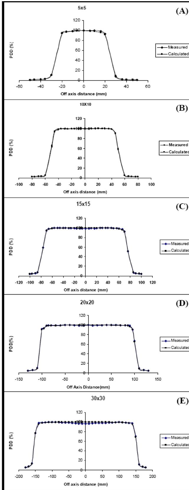
Figure 11 : Measured cross-beam profiles for 6 MV photon beam emerged from Elekta Precise™ linac. at depth  $d_{max}$  compared with calculated one for field size: (A) 5x5 cm<sup>2</sup>, (B) 10x10 cm<sup>2</sup>, (C) 15x15 cm<sup>2</sup>, (D) 20x20 cm<sup>2</sup> and (E) 30x30 cm<sup>2</sup>.
