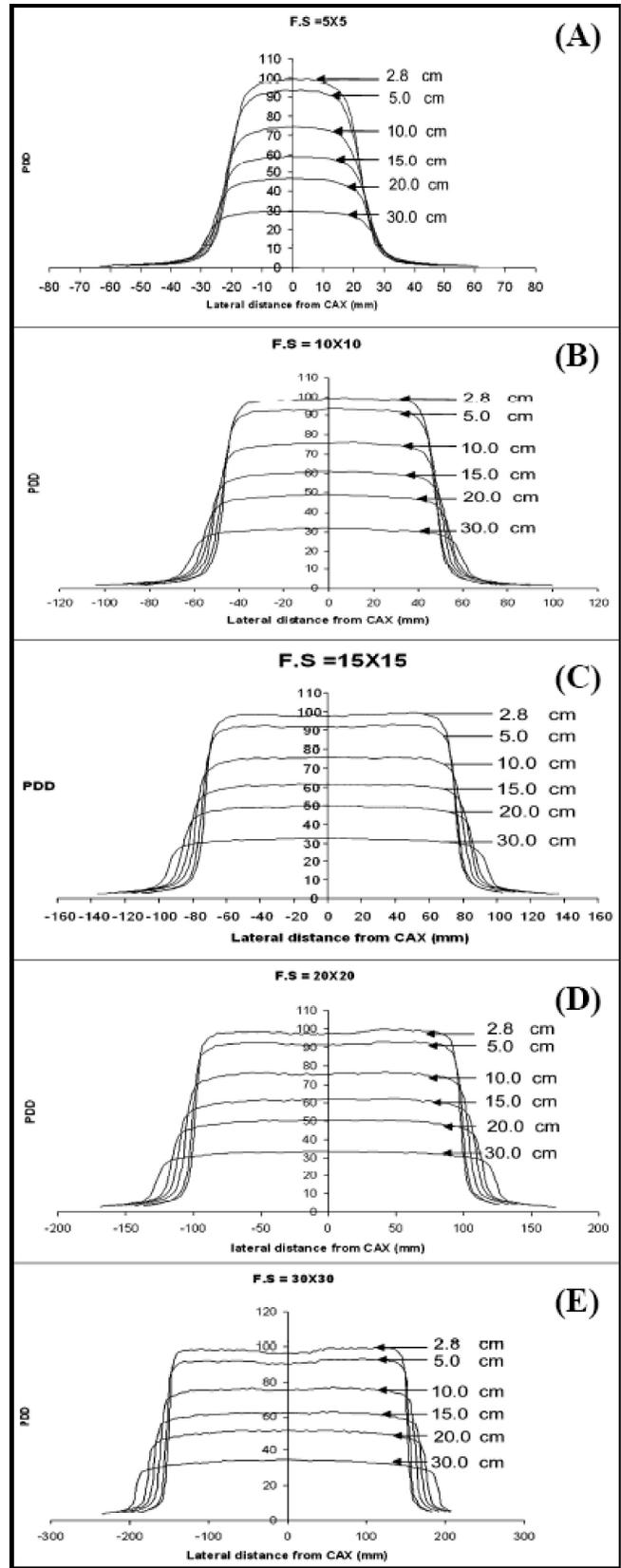
Figure 3 : 6 MV beam profile of Elekta Precise™ linac. scans at depths of (1.6, 5, 10, 15, 20, and 30 cm) for field size: (A) 5x5 cm<sup>2</sup>, (B) 10x10 cm<sup>2</sup>, (C) 15x15 cm<sup>2</sup>, (D) 20x20 cm<sup>2</sup> and (E) 30x30 cm<sup>2</sup>
