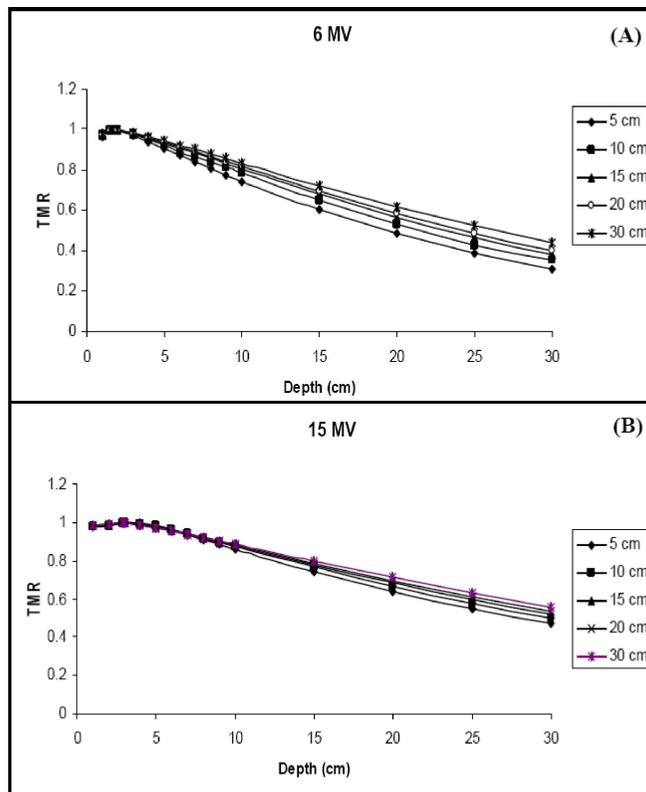
**Figure 7 :** The TMR of photon beam emerged from Elekta Precise™ linac for square fields of sides 5, 10, 15, 20 and 30 cm at FSD = 100 cm, for beam energies (A) 6MV and (B) 15 MV.
