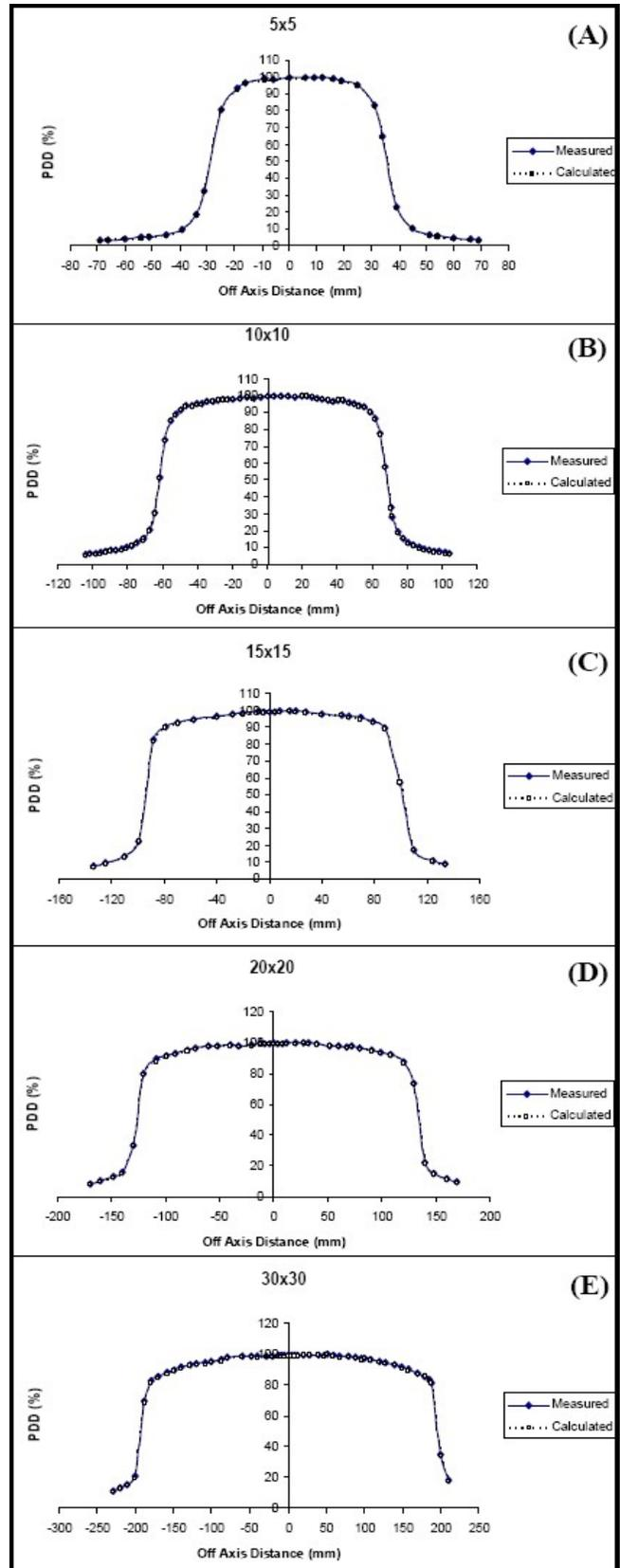
Figure 12 : Measured cross-beam profiles for 15 MV photon beam emerged from Elekta Precise™ linac. at depth  $d_{max}$  compared with calculated one for field size: (A) 5x5 cm<sup>2</sup>, (B) 10x10 cm<sup>2</sup>, (C) 15x15 cm<sup>2</sup>, (D) 20x20 cm<sup>2</sup> and (E) 30x30 cm<sup>2</sup>.
