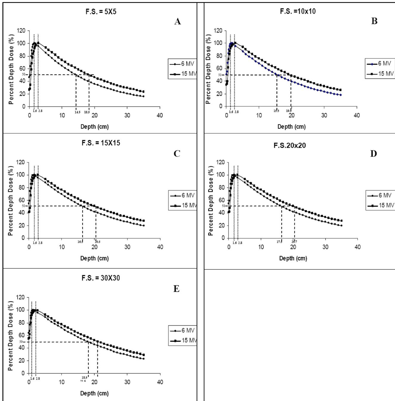
Figure 2 : The central axis PDD curves for 6 MV and 15 MV photon beams of Elekta Precise™ linac. normalized to 100% at  $d_{max}$  for field size: (A) 5x5 cm<sup>2</sup>, (B) 10x10 cm<sup>2</sup>, (C) 15x15 cm<sup>2</sup>, (D) 20x20 cm<sup>2</sup> and (E) 30x30 cm<sup>2</sup>.
