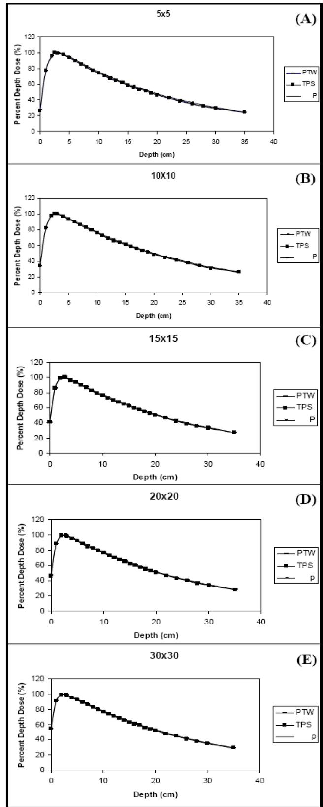
Figure 10 : Measured PDD for 15 MV photon beam emerged from Elekta Precise™ linac. at FSD =100cm in water phantom, compared with calculated and published<sup>[6]</sup> PDD. of open square field size: (A) 5x5 cm<sup>2</sup>, (B) 10x10 cm<sup>2</sup>, (C) 15x15 cm<sup>2</sup>, (D) 20x20 cm<sup>2</sup> and (E) 30x30 cm<sup>2</sup>.
