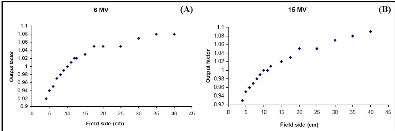
Figure 8 : The output factors for different field sizes relative to field size of a (10x10) cm<sup>2</sup> at depth d<sub>max</sub> cm for photon beam emerged from Elekta Precise™ linac with energy (A) 6MV and (B) 15 MV
