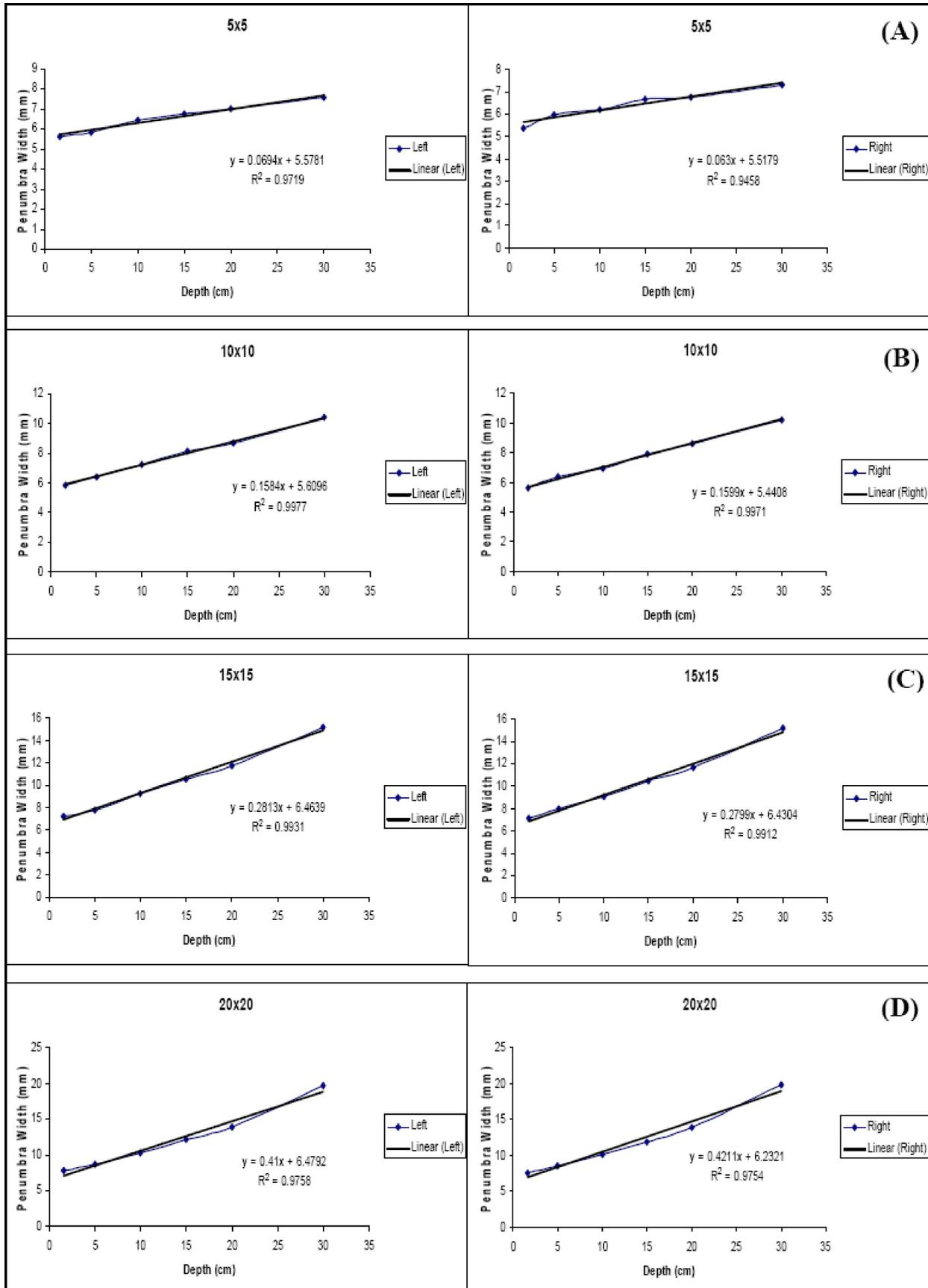
Figure 5 : The linearity between penumbra width and depth for 6MV photon beam emerged from Elekta Precise™ linac. with field size : (A) 5x5 cm<sup>2</sup>, (B) 10x10 cm<sup>2</sup>, (C) 15x15 cm<sup>2</sup>, (D) 20x20 cm<sup>2</sup>
