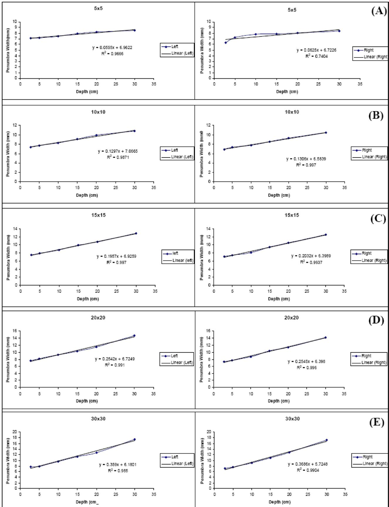
Figure 6 : The linearity between penumbra width and depth for 15 MV photon beam emerged from Elekta Precise™ linac. with field size : (A) 5x5 cm<sup>2</sup>, (B) 10x10 cm<sup>2</sup>, (C) 15x15 cm<sup>2</sup>, (D) 20x20 cm<sup>2</sup> and (E) 30x30 cm<sup>2</sup>.
