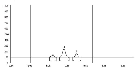
Fig. 4: Densitogram of acid (1N HCl, reflux for 2 h, temp 70°C) treated drug; peak 1 (degraded) (R<sub>f</sub> : 0.35), peak 2 (degraded) (R<sub>f</sub> : 0.47), peak 3 (Standard) (R<sub>f</sub> : 0.625)
