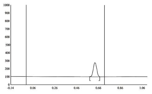
Fig. 2. Densitogram of standard drug (100 ng); peak 1 ( $R_f$ : 0.61 ± 0.02) measured at 232 nm, mobile phase chloroform : methanol (9.8 : 0.2 v/v)
