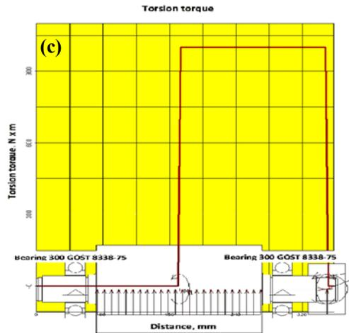
a - Bending torque in vertical plane; b - Bending torque in horizontal plane; c – Torsion torque
