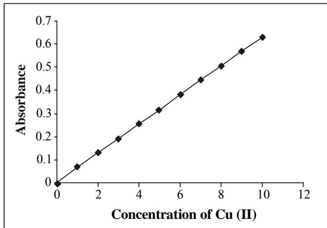
**Fig. 1: Calibration plot of Cu (II): HCHNM complex**
