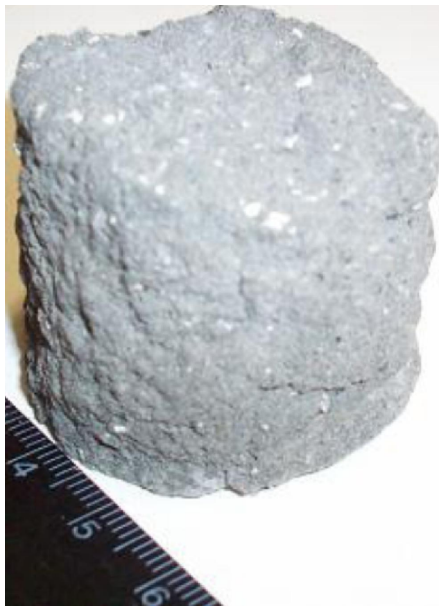
Figure 8 : Typical cement sample reinforced with 34% recyclable materials (17% water treated crumb rubber and 17% flakes).
