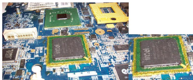
Figure 9 : Typical reworked PCB showing a BGA (black region surrounded by the green region) on top of the (yellow) latex gelatinous stencil.
