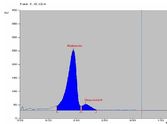
Figure 7 : Chromatogram of Rutoside subjected to light degradation
