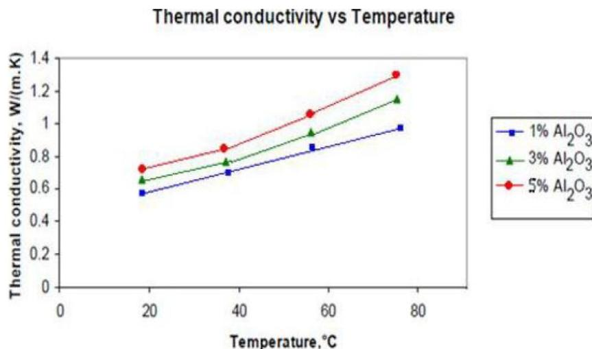
Figure 5 : Thermal conductivity Vs temperature graph of  $\text{Al}_2\text{O}_3$  nanofluids
