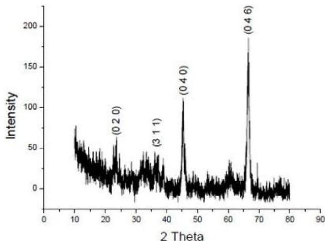
Figure 4 : XRD of aluminium oxide nanopowder
