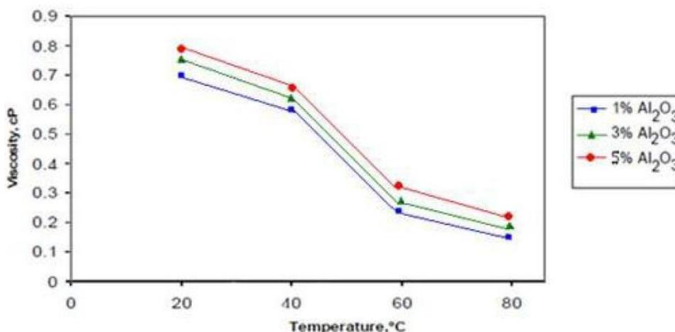
Figure 6 : ViscosityVs Temperature graph of Al<sub>2</sub>O<sub>3</sub> nanofluid
