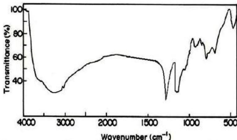
Figure 1 : FT-IR spectra of aluminium oxide nanofluid
