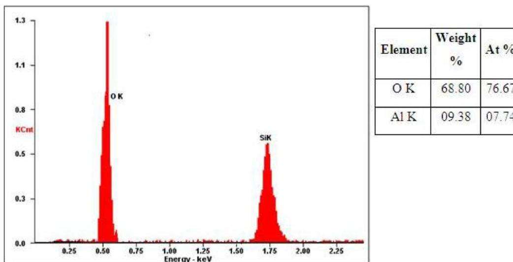
Figure 3 : EDS of aluminium oxide nanopowder
