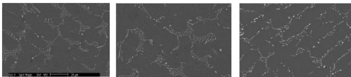
After 50 hours at 1,000°C; After 50 hours at 1,100°C; After 50 hours at 1,200°C Figure 1: Microstructures after 50 hours at 1,000, 1,100 or 1,200°C (SEM pictures in BSE mode)
