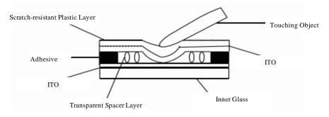
Figure 2 : Structure of resistive touch screen
