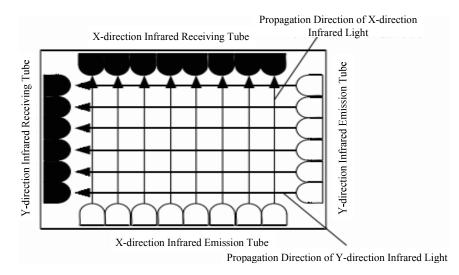
**Figure 4 : Structure of infrared touch screen**
