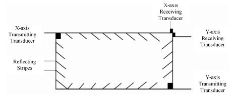
Figure 3 : Structure of surface acoustic wave touch screen
