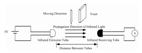
**Figure 6 : Structure of testing device**
