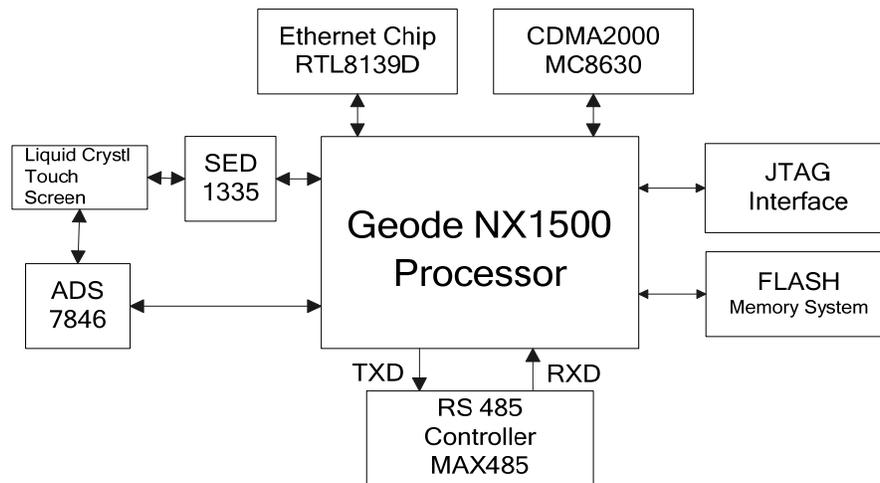
Figure 2 : Embedded-based system of intelligent home hardware platform structure
