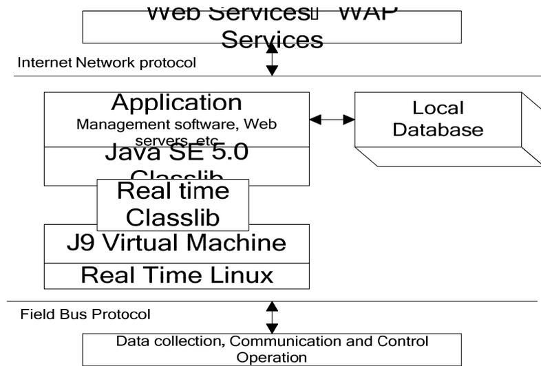
Figure 3 : The structure diagram of intelligent home gateway
