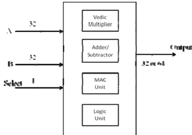
**Fig. 6: Arithmetic logic unit**
