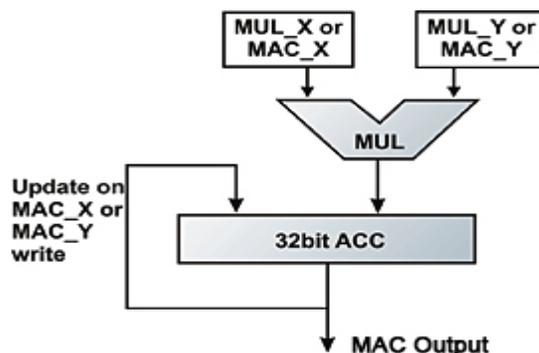
Fig. 4: Multiply and accumulate unit
