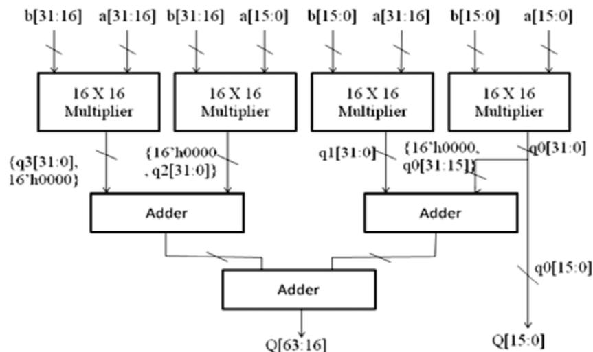
Fig. 3: Block diagram of 32 x 32 multiply block
