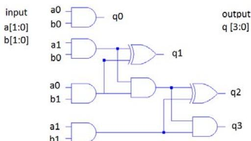
**Fig. 2: Hardware realization of 2 x 2 block**
