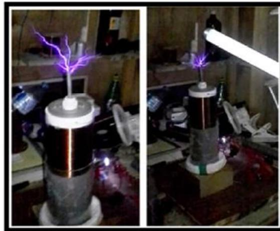
**FIG. 4. Corona (left) and glowing a fluorescent light wirelessly (right).**
