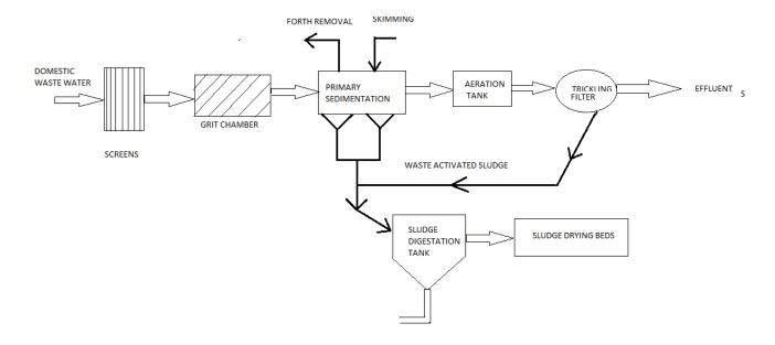
FIG. 1. Waste water treatment plant flow diagram.
