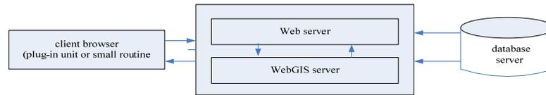
**Figure 3 : Three-layer system structure of WebGIS**
