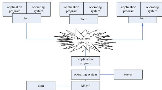
**Figure 2 : C/S two-layer structure system diagram**
