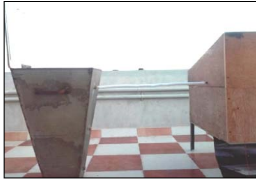
Fig. 3: Integration of solar still and solar pond on UCZ
