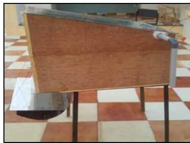
Fig. 1: Fabrication of solar still
