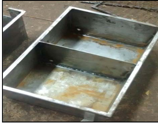
Fig. 3: Outer casing of water tank
