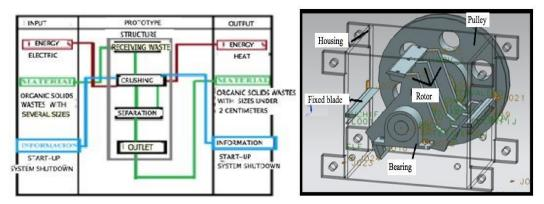
FIG. 4. Service functions and their interrelationships [8]. FIG. 5. 3D model of crushing machine
