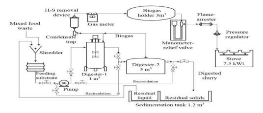
FIG. 1. Overview diagram of the biogas plant [2].
