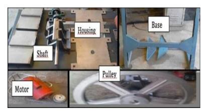
FIG. 6. Pieces of the crushing machine
