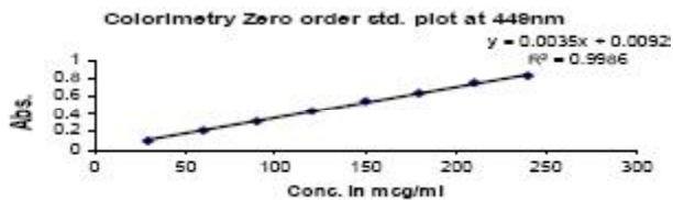
Figure 3 : Calibration curve of metadoxine in distilled water with ferric nitrate reagent for zero order
