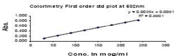
Figure 4 : Calibration curve of metadoxine in distilled water with ferric nitrate reagent for first order
