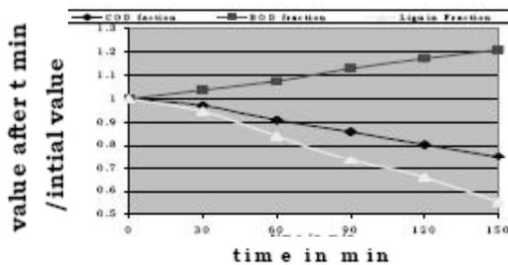
Figure 8 : Plot of fraction of  $V_t/V_0$  against time during degradation studies in presence of UV light, Catalyst, Peroxide
