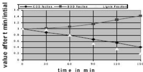
Figure 6: Plot of fraction of  $V_t/V_0$  against time during degradation studies in presence of UV light, air, Catalyst, Peroxide
