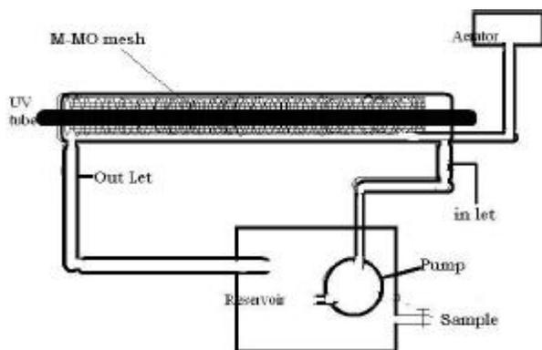
Figure 2: Design of photo-catalytic reactor
