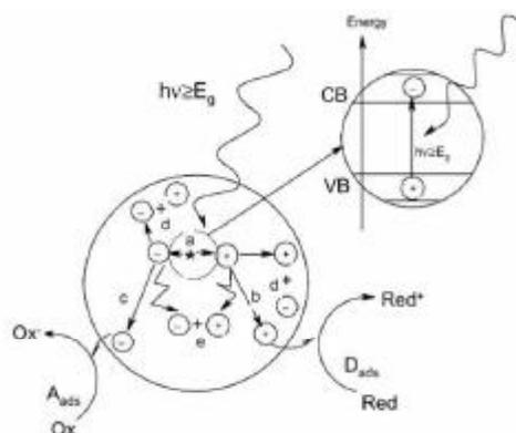
Figure 1: Mechanism of photo catalysis
