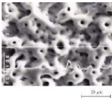
Figure 3: Topography of oxide film formed
