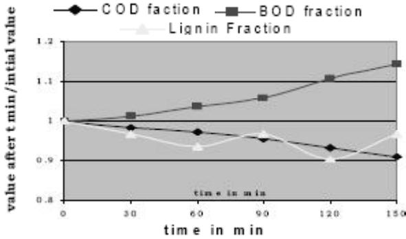
Figure 7: Plot of fraction of  $V_t/V_0$  against time during degradation studies in presence of air, Catalyst, Peroxide
