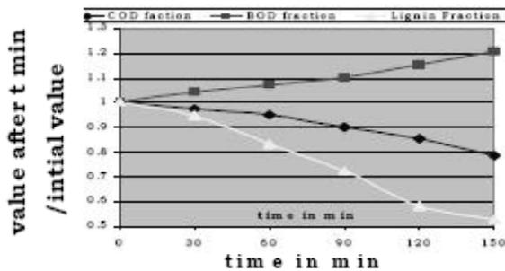
Figure 9: Plot of fraction of  $V_t/V_0$  against time during degradation studies in presence of UV light, air, peroxide
