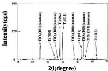
Figure 4: XRD pattern of Ti-O layer
