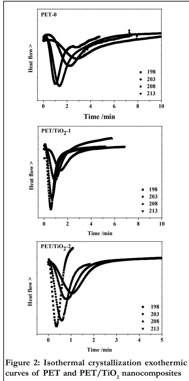
Figure 2: Isothermal crystallization exothermic curves of PET and PET/ $TiO_2$  nanocomposites
