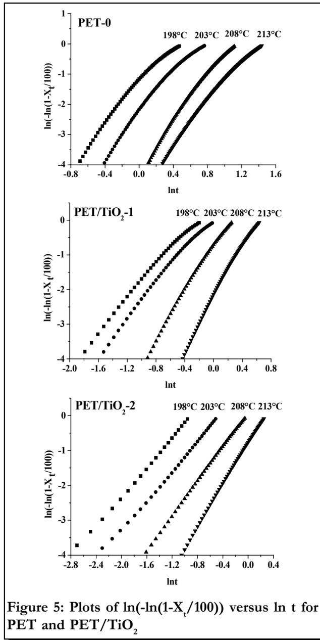
Figure 5: Plots of ln(-ln(1-X<sub>t</sub>/100)) versus ln t for PET and PET/TiO<sub>2</sub>
