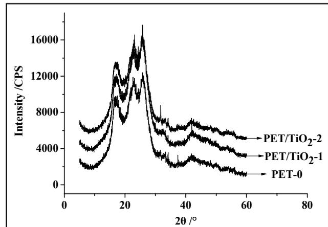
**Figure 7: WAXS diffraction of neat PET and PET/TiO<sub>2</sub> composites**
