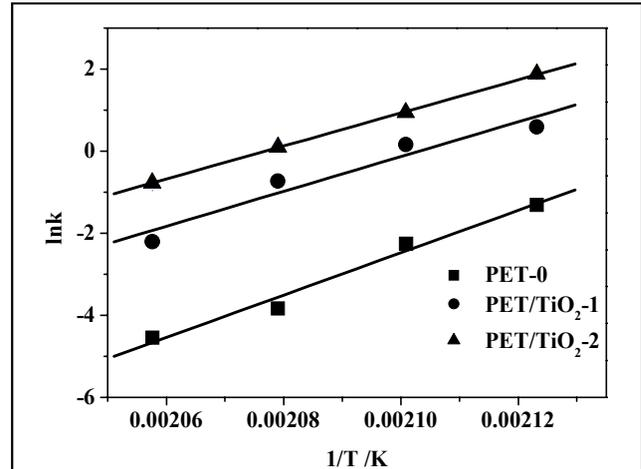
**Figure 6: Change of activation energy of the overall crystallization with crystallization temperatures**
