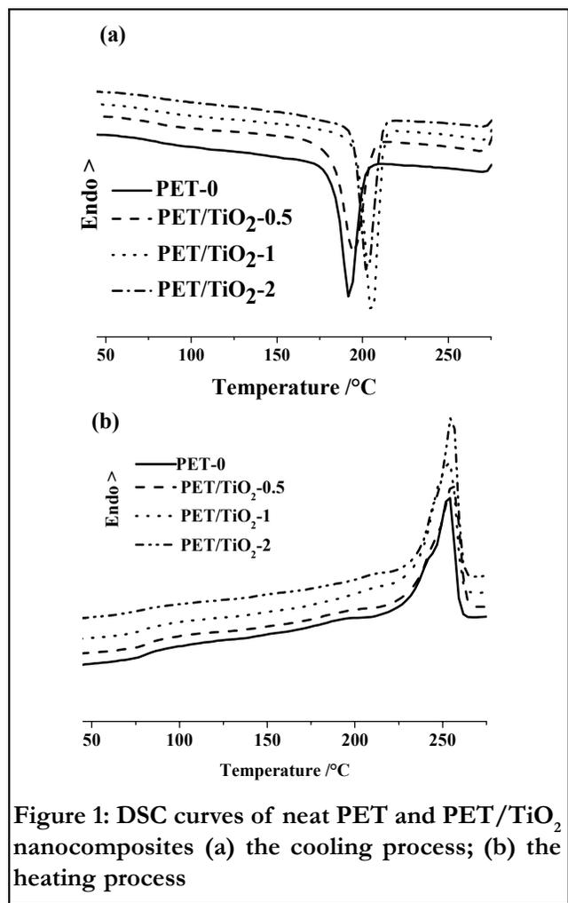
Figure 1: DSC curves of neat PET and PET/TiO<sub>2</sub> nanocomposites (a) the cooling process; (b) the heating process
