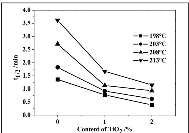
Figure 4: Relationship between t<sub>1/2</sub> and content of TiO<sub>2</sub>
