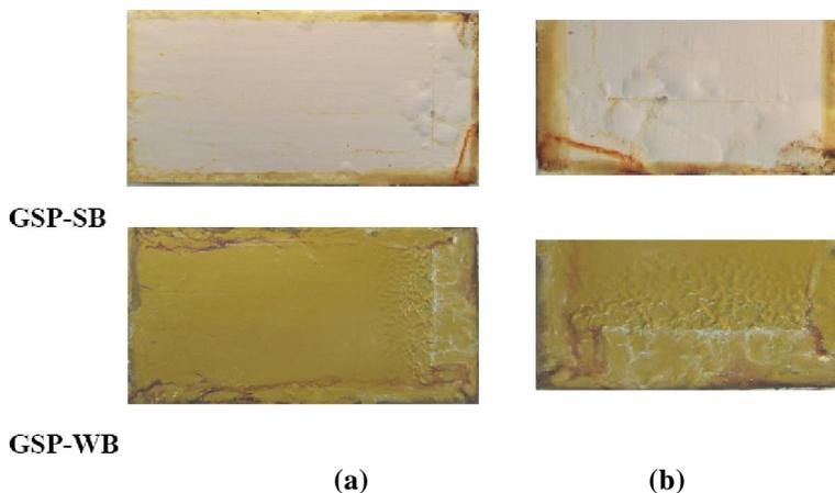
Figure 2 : Final condition of the samples after the exposure in the SSC; (a) global view and (b) detail of the incision area
