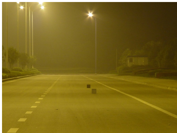
Figure 3 : In road or tunnel lighting environment, the small target of the negative contrast is easy to be indented than positive contrast
