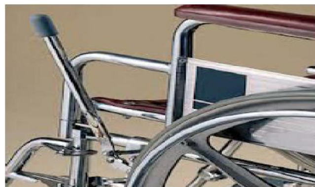
Figure 2 : Brake system of a smart wheelchair
