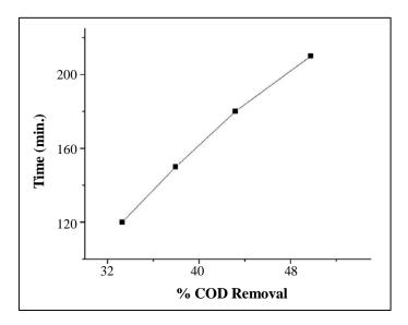
Fig. 4: Effect of reaction time on COD removal
