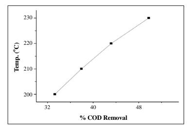
Fig. 2: Effect of temperature on COD removal
