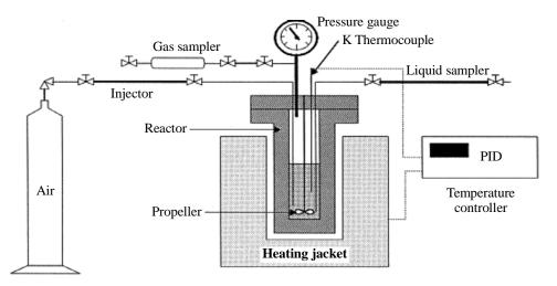
Fig. 1: Thermal liquid-phase oxidation process unit (Basic flow diagram)
