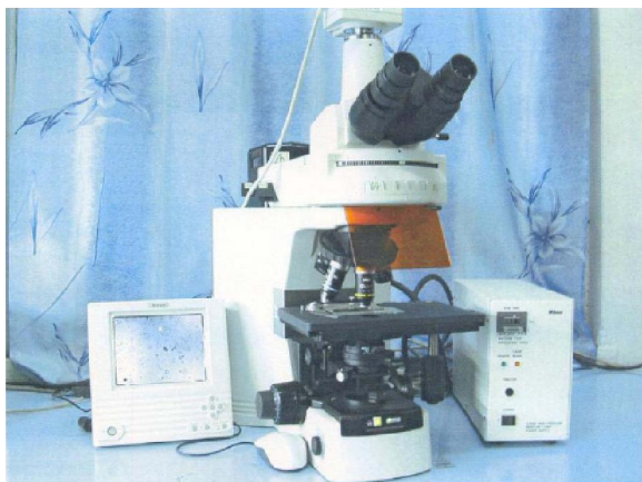
Figure 1 : A view of trinocular microscope (Make: Nikon, Japan) used for examination and identification of house dust mites
