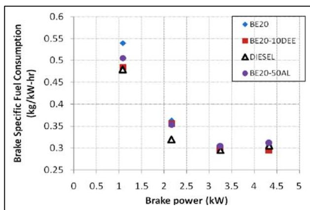
**Fig. 4: Variation of brake specific fuel consumption with load**
