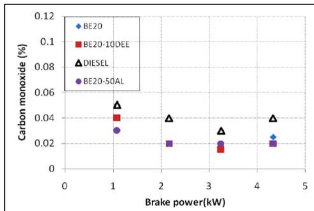
**Fig. 6: Variation of carbon monoxides with load**
