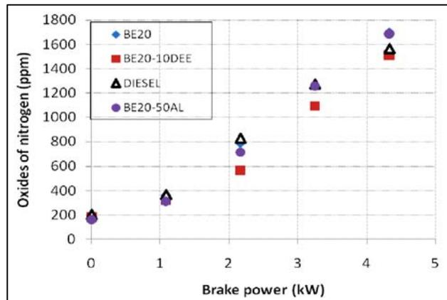
**Fig. 5: Variations of oxides of nitrogen with load**
