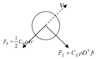
Figure 2: Table tennis force schematic diagram
