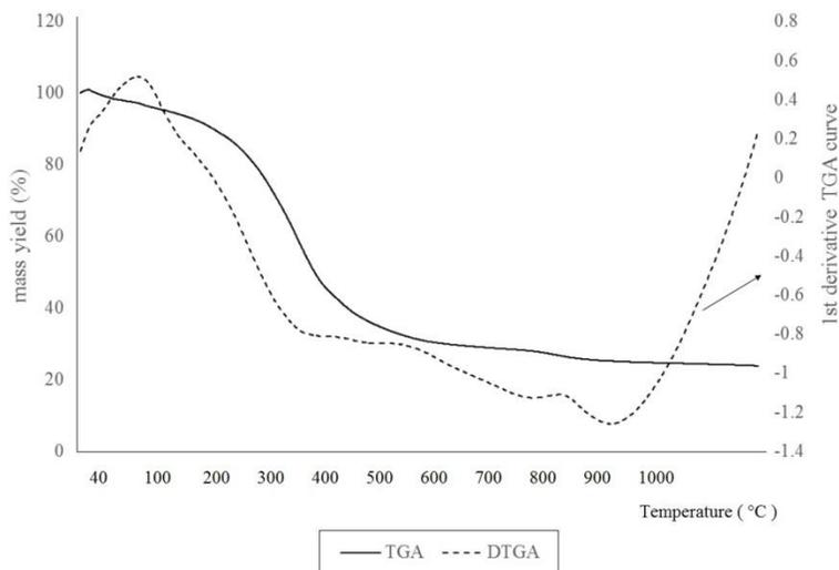
FIG. 4. Thermogravimetric analysis (TGA) of dried food waste.
