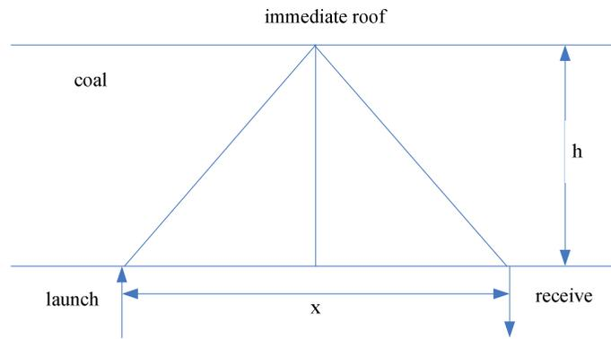
Figure 1 : The schematic diagram of the elastic wave detecting top-coal thickness
