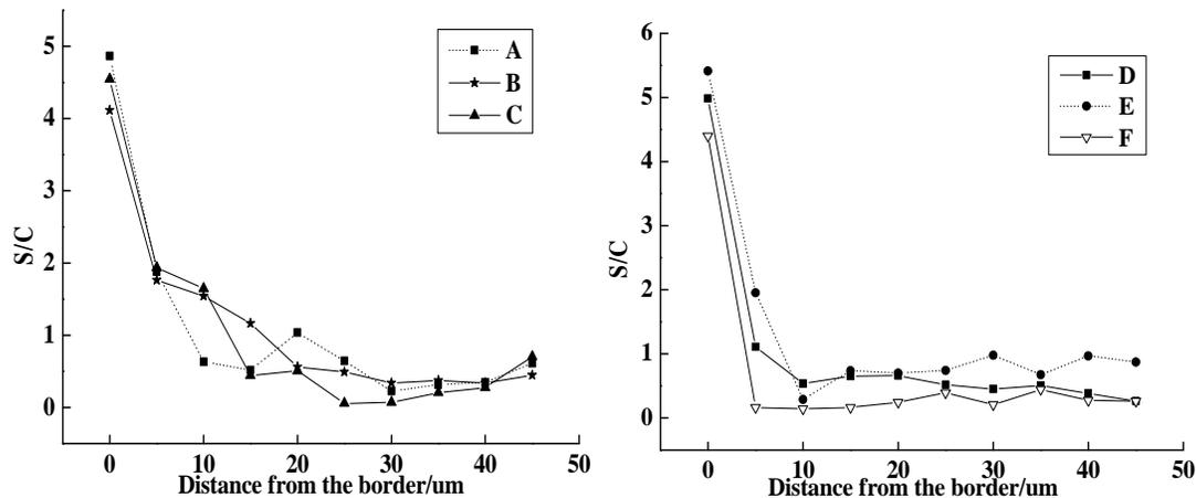
Figure 6 Silica/calcium oxide (S/C) mass ratio in interfacial transition zone
