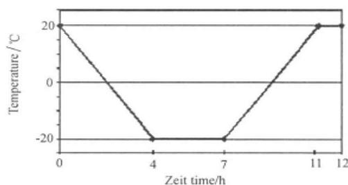
Figure 1 Freezing-thawing cycle of CDF test
