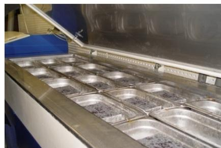
Figure 2 Experimental device for one-side freeze-thaw
