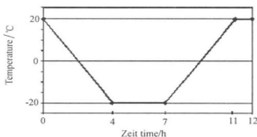
Figure 1 Freezing-thawing cycle of CDF test
