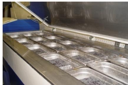
Figure 2 Experimental device for one-side freeze-thaw
