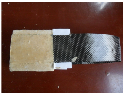
Figure 2 The double shear test specimen used to affix the sheet
