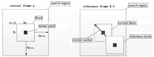
Figure 1 : The diagram for relative movement of current block and matching block
