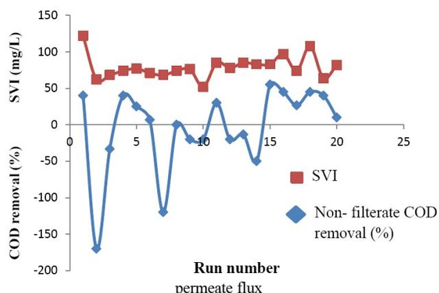
Figure 7 : Non-filtrate COD removal (%) and SVI vs. run number
