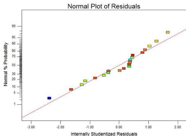
**Figure 3 : Normal probability plot of residual for COD removal (%)**
