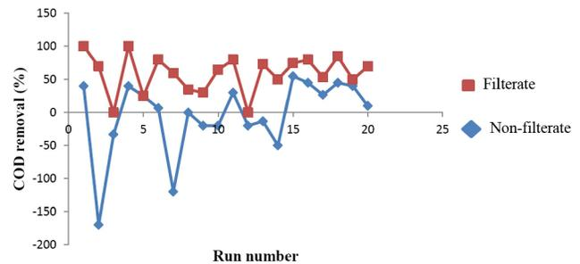
Figure 5 : Comparison between filtrate and non-filtrate COD removal (%)
