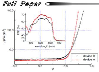
Figure 4 : Effect of donor layer (PCBM) on performance of polymer solar cells: current–voltage (J - V) characteristics of reference device B (black circle) with the structure ITO/ PEDOT-PSS/P3HT: PCBM/Ca/Al and for device A (red uptriangle) with the structure ITO/PEDOT-PSS/P3HT:PCBM/ Ca/Al. Inset shows the EQE measurements for device A and reference device B.
