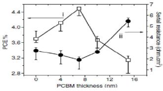
Figure 2 : Effect of PCBM thickness on device performance: plot shows power conversion efficiency (open squares, curve i) and series resistance (fill circles, curve ii) for different thicknesses of PCBM layer annealed at 110 °C for 30 min in device A. Device area was 0.12 cm2.
