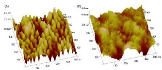
Figure 3 : Effect of annealing on morphology of top PCBM layer: AFM height images of device A showing a 500 nm  $\times$  500 nm surface area. (a) Unannealed 7 nm PCBM layer; (b) 7 nm PCBM layer annealed at 110 °C for 30 min. Scale on *z* axis = 5 nm.
