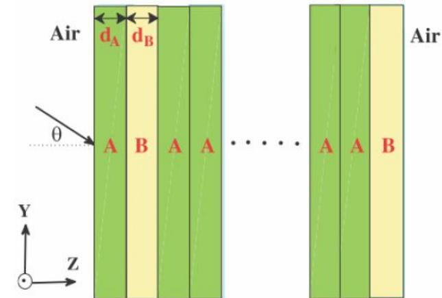
Figure 1 : Schematic drawing of the one-dimensional quasiperiodic Fibonacci structure, which is embedded in air. The thicknesses of A and B are supposed to be  $d_A$  and  $d_B$ , respectively.
