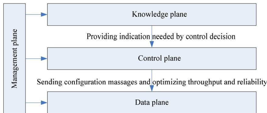
Figure 2 : Independent system architecture of IOT
