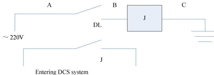
Figure 3 : Isolation cabinet function diagram
