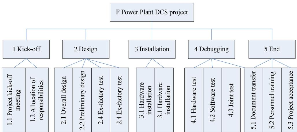
**Figure 4 : Work breakdown structure of F power plant DCS project**
