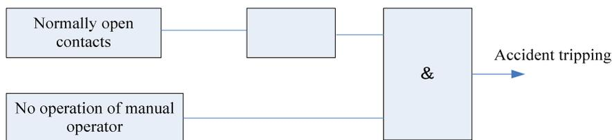
**Figure 1 : Accident tripping logics of electrical switch**
