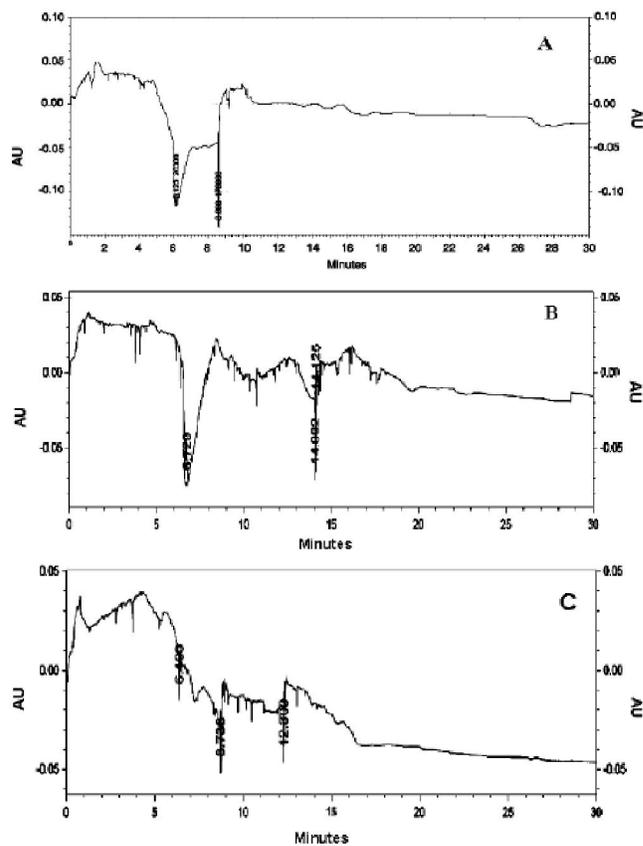
Figure 4 : (A) Electropherogram obtained by micellar electrokinetic chromatography for UDP-glucose ( $1.0\text{ mg mL}^{-1}$ ) used as standard. (B): Electropherogram obtained by micellar electrokinetic chromatography for UDP-glucuronic acid ( $1.0\text{ mg mL}^{-1}$ ) used as standard. (C) Electropherogram obtained by micellar electrokinetic chromatography of a mixture of UDP-glucose and UDP-glucuronic acid ( $1.0\text{ mg mL}^{-1}$ ) used as standards. Detection was monitored at 214 nm.
