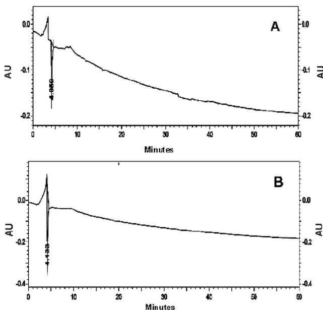
Figure 2 : (A) Electropherogram obtained by capillary electrophoresis with indirect detection and reversion of the polarity for UDP-glucose ( $0.5\text{ mg mL}^{-1}$ ) used as standard. (B): Electropherogram obtained by capillary electrophoresis technique with indirect detection and reversion of the polarity for UDP-glucuronic acid ( $0.5\text{ mg mL}^{-1}$ ) used as standard. Detection was monitored at 214 nm.
