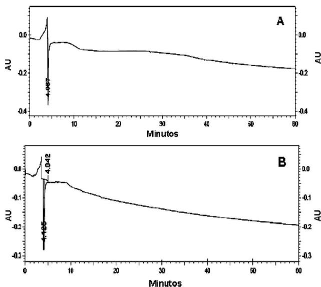
Figure 1 : (A) Electropherogram obtained by capillary electrophoresis with indirect detection and reversion of the polarity for UDP-glucose ( $1\text{ mg mL}^{-1}$ ) used as standard. (B) Electropherogram obtained by capillary electrophoresis with indirect detection and reversion of the polarity for UDP-glucuronic acid ( $1\text{ mg mL}^{-1}$ ) used as standard. Detection was monitored at 214 nm.
