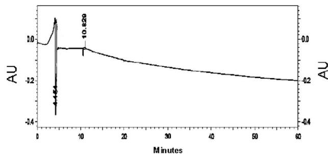
Figure 3 : Electropherogram obtained by capillary electrophoresis with indirect detection and reversion of the polarity of a mixture of UDP-glucose and UDP-glucuronic acid ( $0.5\text{ mg mL}^{-1}$  each one) used as standards. Detection was monitored at 214 nm.
