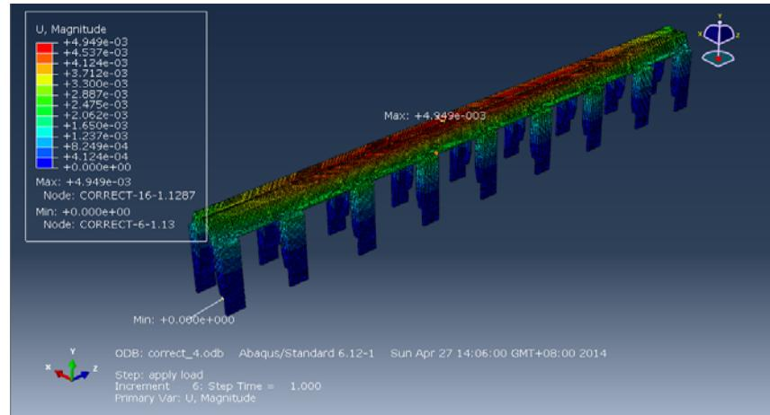
**Figure 7 : The resultant displacement nephogram(optimized)**
