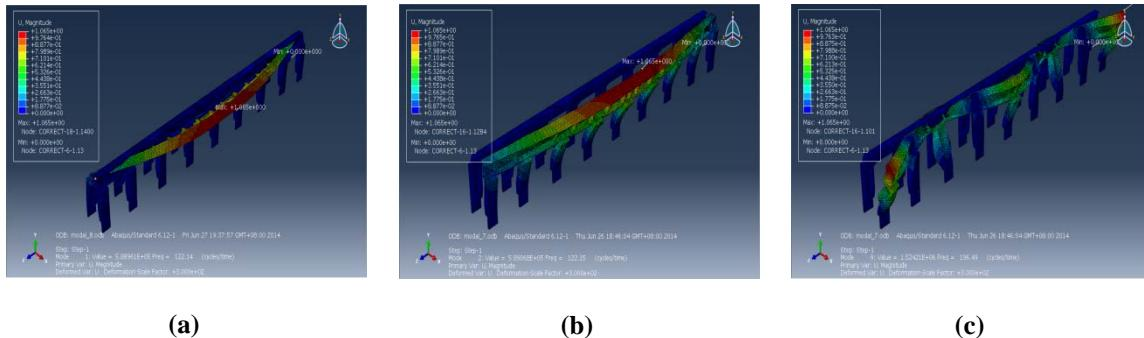
**Figure 10 : The vibration modes, (a)-The first vibration mode, (b)-The second vibration mode, (c)-The ninth vibration mode**
