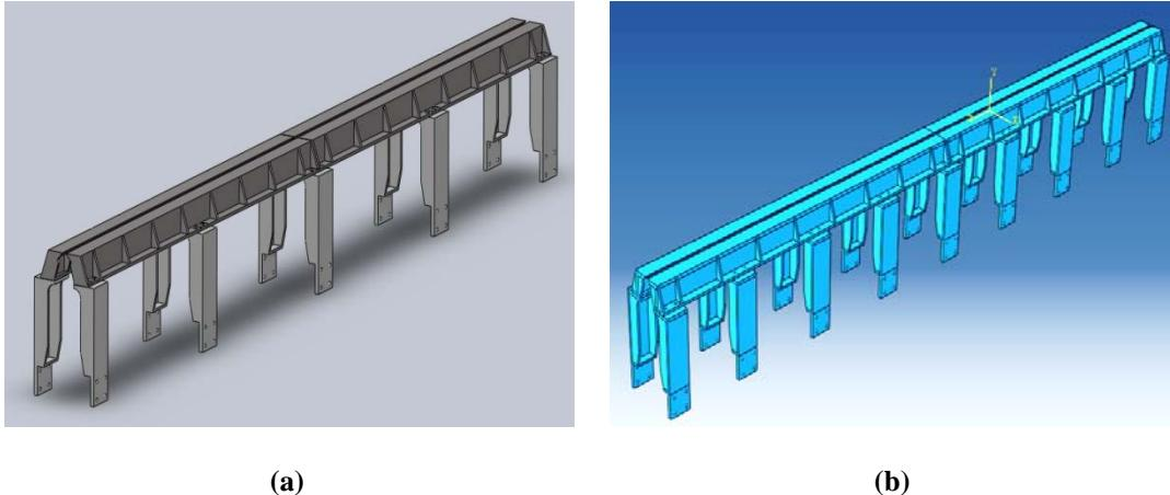
**Figure 6 : The main structure of grating scale copy machine, (a)-The original structure, (b)-The optimized structure**
