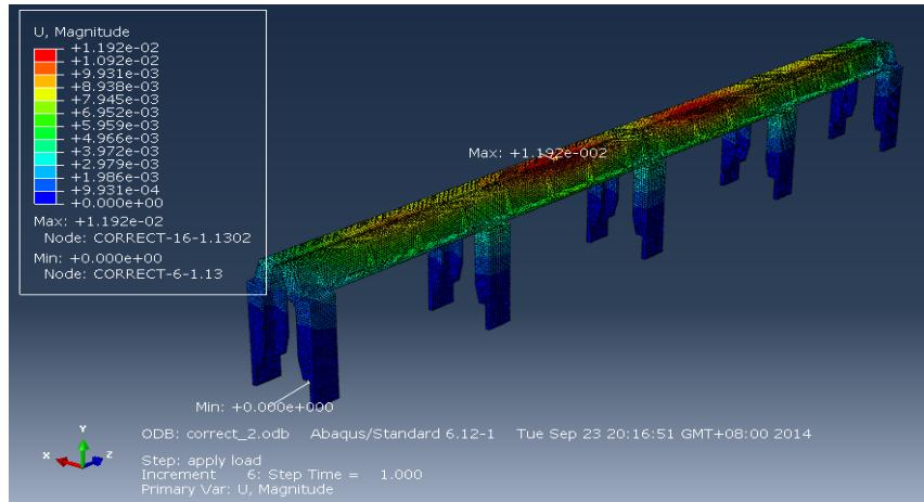
**Figure 3 : The resultant displacement nephogram(original)**
