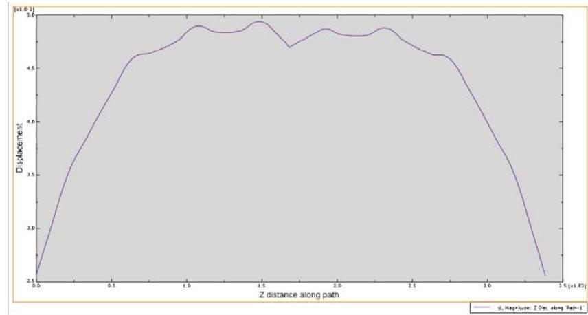
**Figure 8 : The graph of resultant displacement along path (optimized)**
