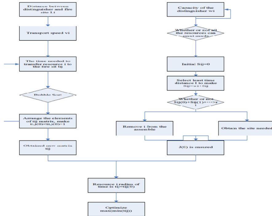
Figure 2: Calculation method of real fire-fighting rescue circle
