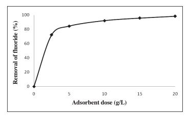
Fig. 3: Effect of dose of activated alumina
