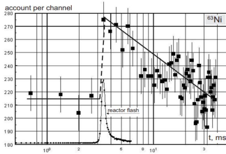
FIG. 2. Result of accumulation of registered beta-electrons emitted by the source  $^{63}\text{Ni}$  [6].
