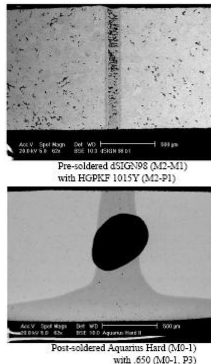
**Figure 2: Internal metallurgical defects in an alloy (micro-shrinkage defects, left hand), in a pre-solder joint (micro-shrinkage defects, left hand) and in a post-solder joint (enormous porosity, right hand)**
