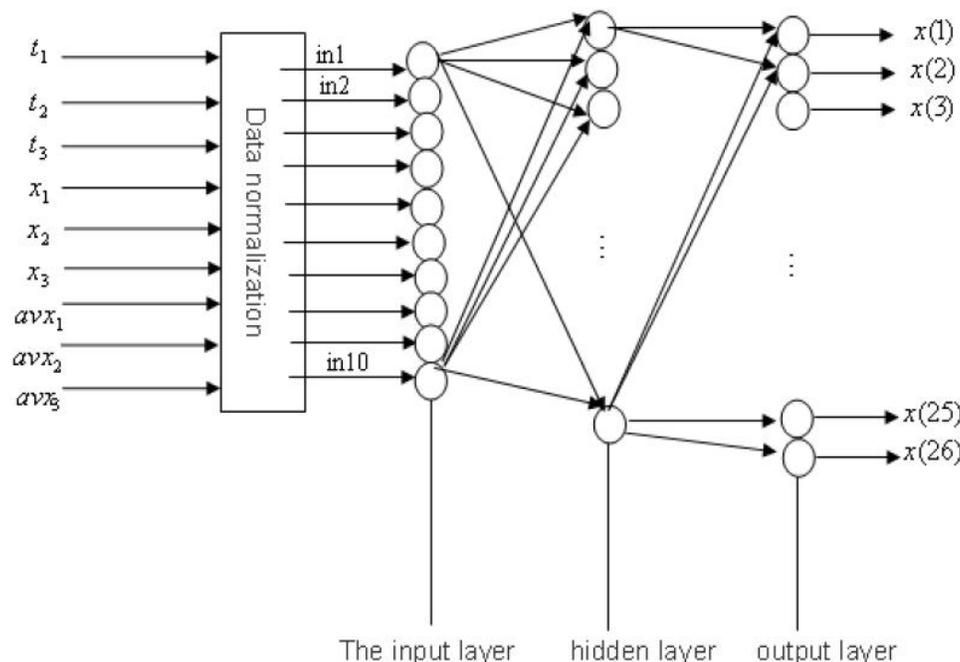
Figure 2 : BP neural network nerve cell structure
