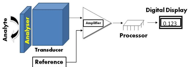
Fig. 1: Schematic diagram with basic components of biosensor
