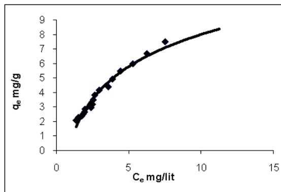
Fig. 1: Adsorption isotherm system: F-300-oxidised carbon-Ni<sup>2+</sup>
