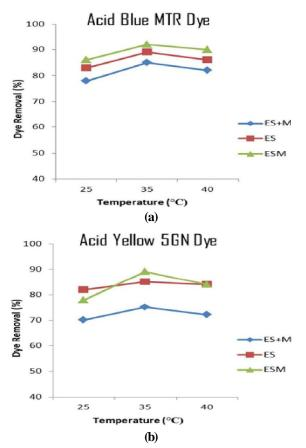
Figure 6 : Effect of temperature on % decolourization of (a) Acid Blue MTR Dye & (b)Acid Yellow 5GN dye by using ES+M,ES and ESM
