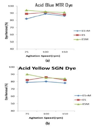
Figure 5 : Effect of agitation on % decolourization of (a) Acid Blue MTR Dye & (b) Acid Yellow 5GN dye by using ES+M, ES and ESM
