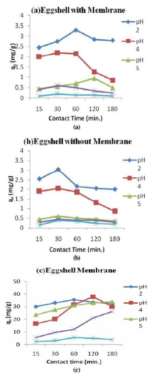
Figure 8 : Plot showing the adsorption kinetics of time vs.  $q_e$  (mg of dye adsorbed per gm of adsorbent) for Acid Blue MTR Dye by using (a) ES+M (b) ES (c) ESM
