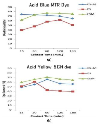
Figure 2 : Effect of contact time on % decolourization of (a) Acid Blue MTR Dye & (b) Acid Yellow 5GN dye by using ES+M,ES and ESM
