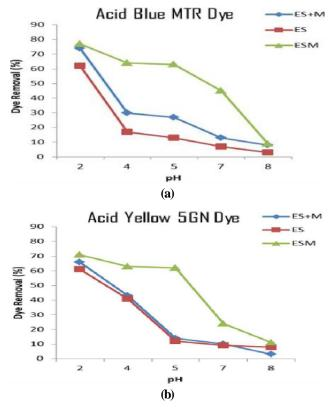
Figure 1 : Effect of pH on % decolourization of (a) Acid Blue MTR Dye & (b) Acid Yellow 5GN dye by using ES+M, ES and ESM
