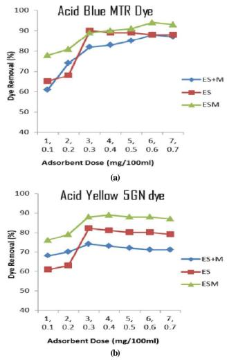
Figure 3 : Effect of adsorbent dosage on % decolourization of (a) Acid Blue MTR Dye & (b) Acid Yellow 5GN dye by using ES+M, ES and ESM
