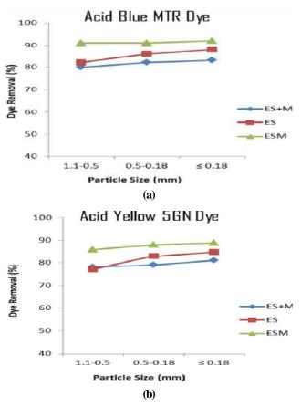
Figure 7 : Effect of particle size on % decolourization of (a) Acid Blue MTR Dye & (b) Acid Yellow 5GN dye by using ES+M, ES and ESM
