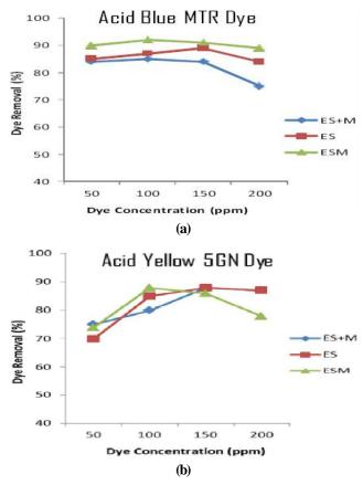
Figure 4 : Effect of dye concentration on % decolourization of (a) Acid Blue MTR Dye & (b) Acid Yellow 5GN dye by using ES+M, ES and ESM
