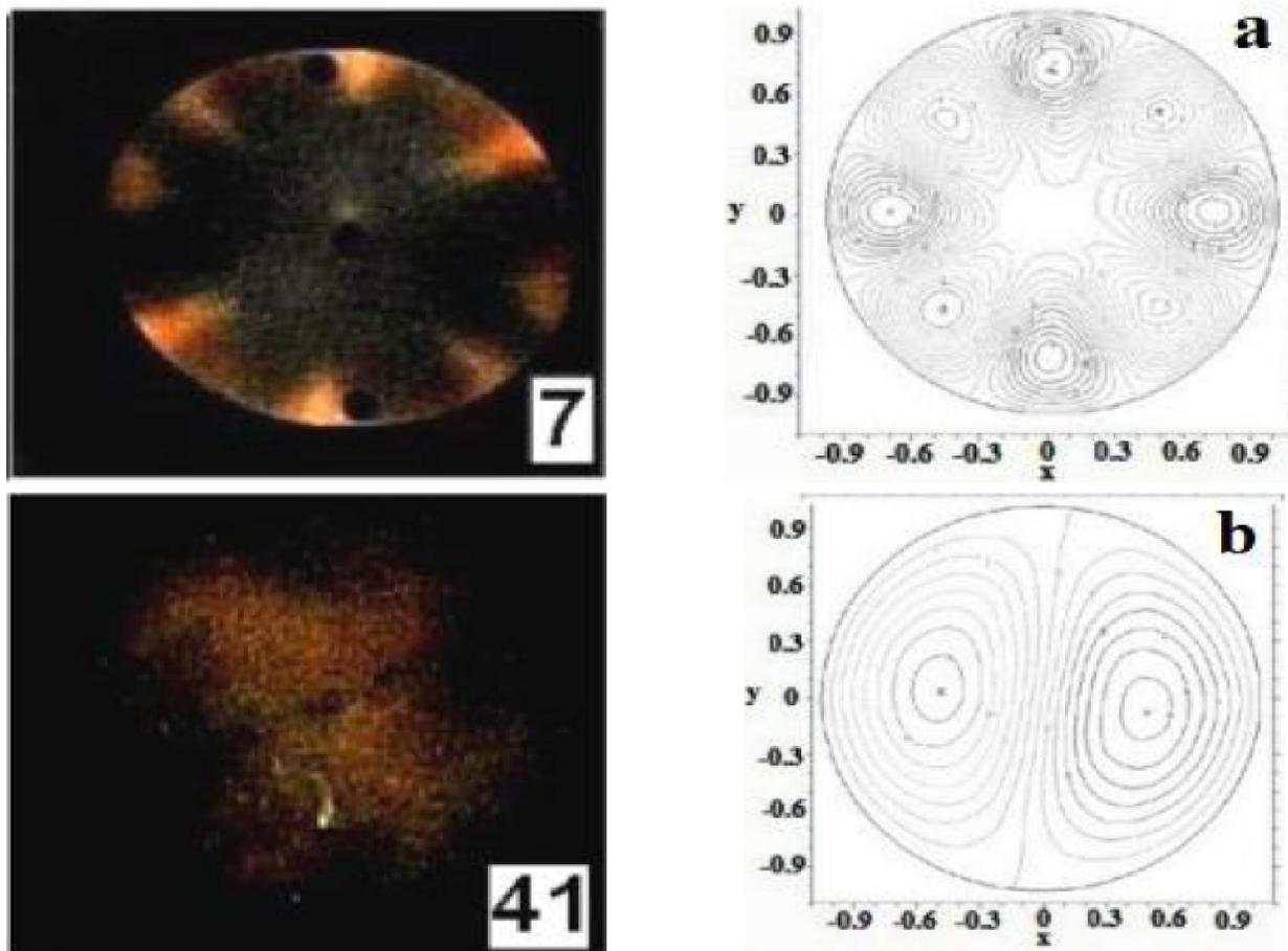
Figure 4 : Frames of video filming from Figure 3c and Figure 3b, and calculated normal modes of vibrations of air in the cylinder, a – the 36<sup>th</sup> mode, b– the 4<sup>th</sup> mode
