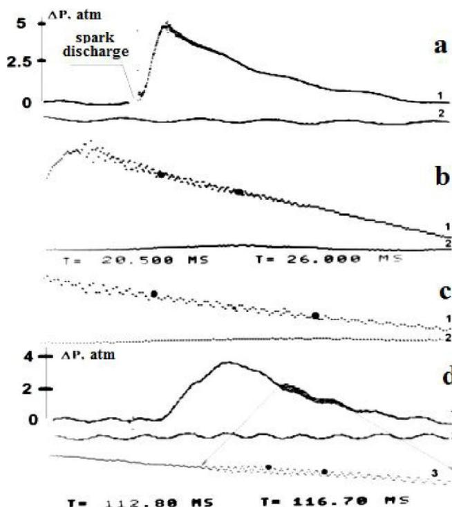
Figure 2 : Oscillograms of pressure change in combustion ignition of gas mixtures; 1 – signal at the initiated ignition; 2 – comparison signal, large black points – time interval; 3 – the stretched time interval; a,b,c –  $(H_2+air)_{stoich}$ , various time intervals; d – 15%  $H_2+air$  + 3%  $CCl_4$
