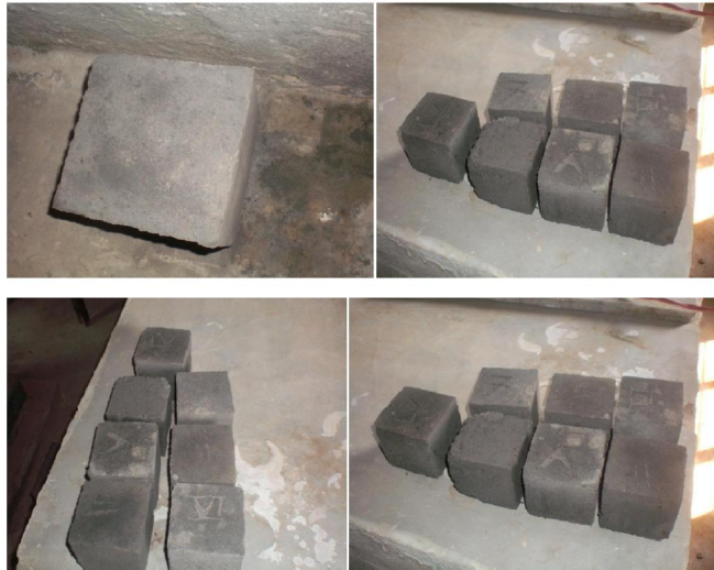
Figure 4 : Concrete cubes made up of fly ash under different conditions
