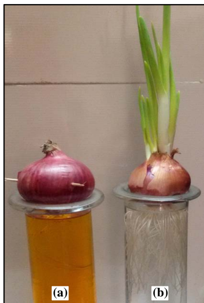
Fig. 1: Growth of onion bulb in (a) orange G and (b) photocatalytically treated solution
